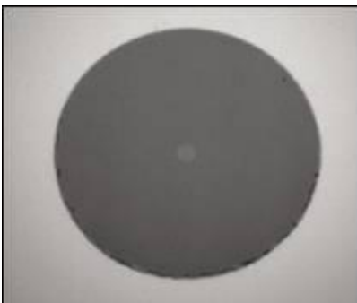
Figure 1. Connector end-face, singlemode fiber, viewed under coaxial illumination, x400. Note small core in the middle.
